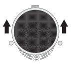
■ Pull the grease filter upwards to remove it.
